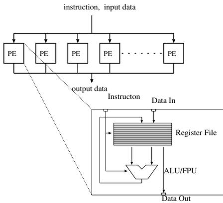
**Figure 2: Basic structure of a SIMD processor**
