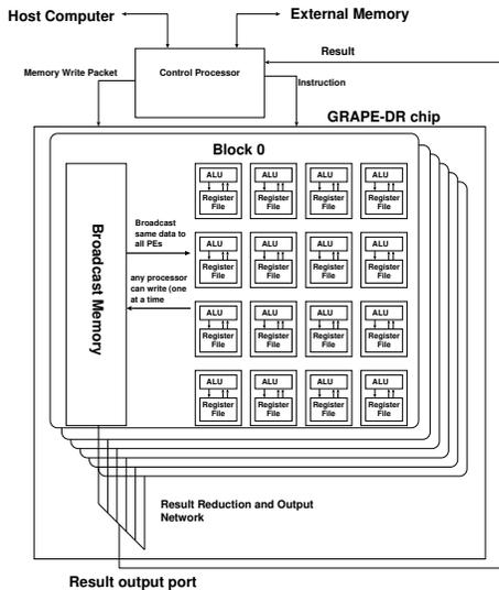
**Figure 6: Overall Architecture of the GRAPE-DR chip**
