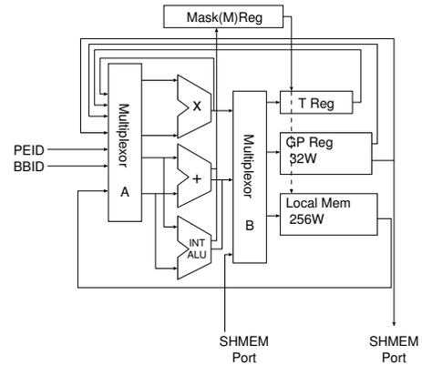
Figure 5: Structure of a Processor Element
