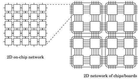
**Figure 3: On-chip two-dimensional network (left) and its extension to multiple chips and multiple boards (right)**
