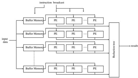
Figure 4: Modified SIMD architecture
