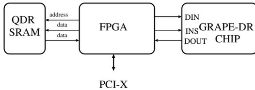
Figure 8: GRAPE-DR chip test board block diagram.
