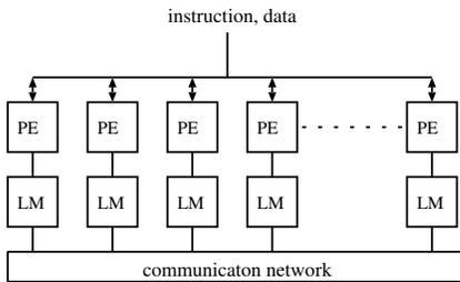
**Figure 1: Structure of a traditional large-scale SIMD processor**
