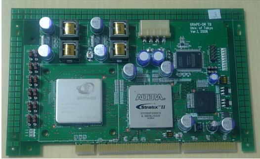
Figure 7: GRAPE-DR chip layout (top) and GRAPE-DR test board (bottom)
