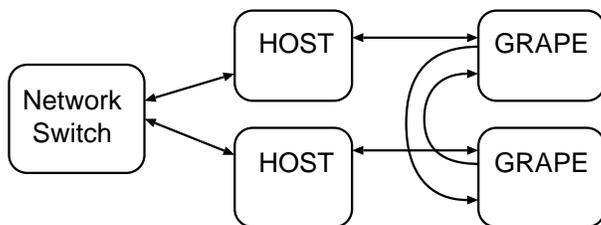
Figure 4: Parallel host with data exchange between GRAPE hardware.
