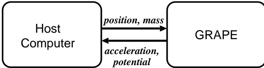
Figure 1: Basic concept of a GRAPE system.
