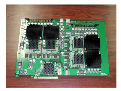
PCIe x16 (Gen 1) interface Altera Arria GX as DRAM controller/communication interface
