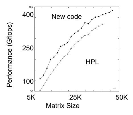
Speed in Gflops as function of Matrix size Top: new code Bottom: HPL 1.04a 430 Gflops (54% of theoretical peak) for N=50K
