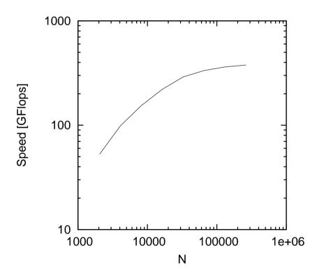
Assembly code (which I wrote) is not very optimized yet... Should reach at least 600 Gflops after rewrite.
