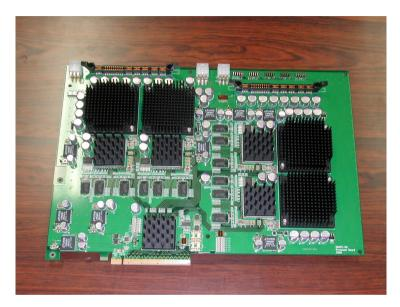
PCIe x16 (Gen 1) interface Altera Arria GX as DRAM controller/communication interface
